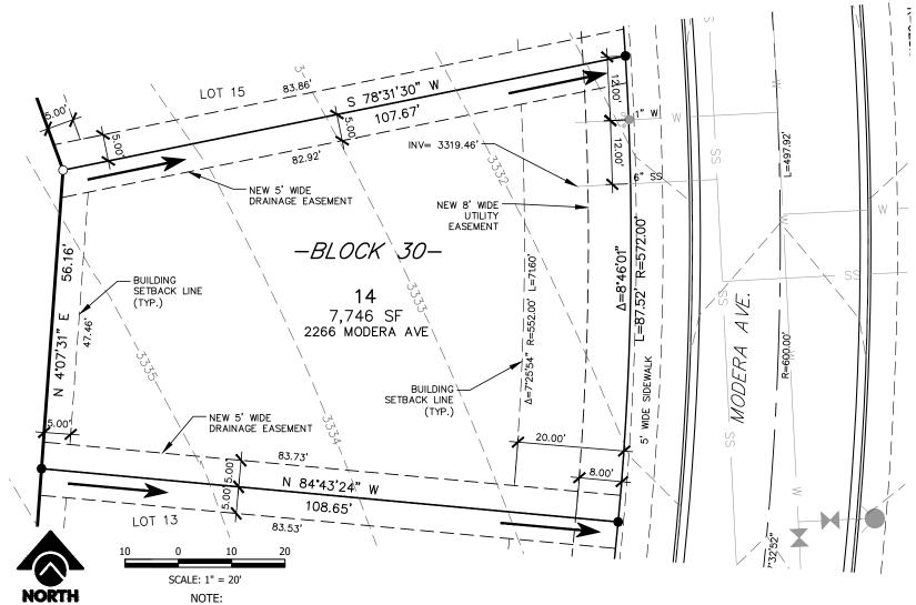
GENERAL DIRECTION OF STORM RUNOFF FROM LOT TO STREET. FINAL GRADING PER BUILDING CODE.
